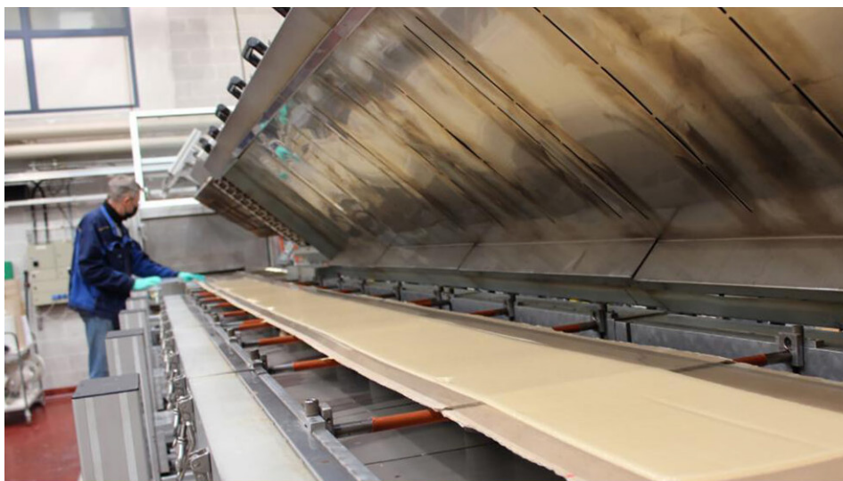
Figure 10: VTT's process to create continuous sheets of mycelium leather. Source: https://www.intelligentliving.co/continuous-sheets-of-mushroom-leather/
