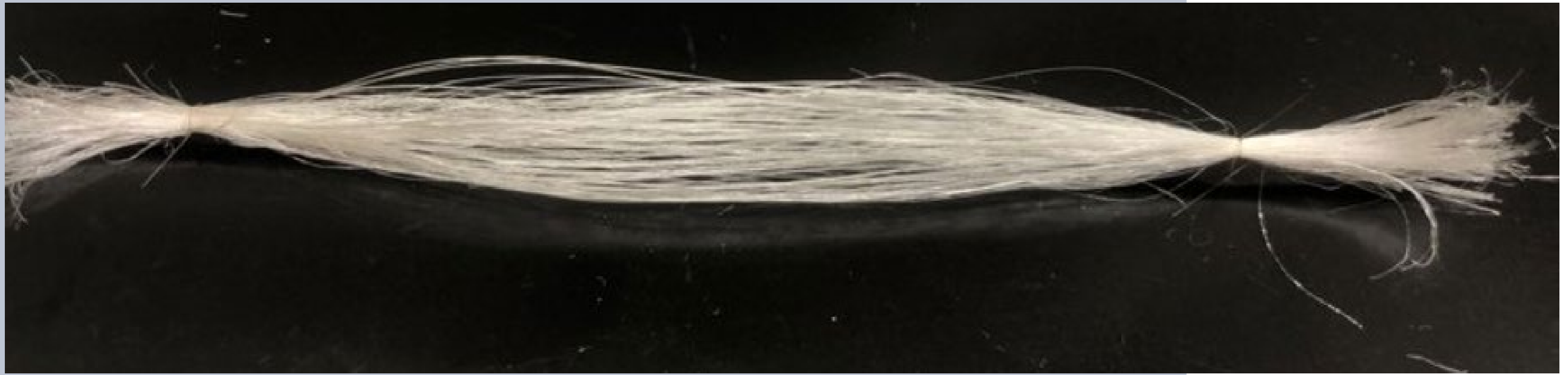
Fig. 5. A bundle of recombinant spider silk protein fiber produced by Dr. Rising's research lab. 49
